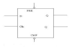
Figure 1: D Flip-Flop Schematic Symbol
