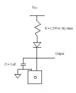
Figure 2: Schematic for Connecting the Switch
