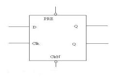
Figure 1: D Flip-Flop Schematic Symbol
