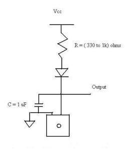
Figure 2: Schematic for Connecting the Switch
