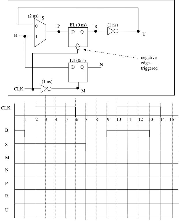
In this circuit, L1 is a positive level-sensitive D latch.
