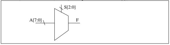
**By drawing the implementation schematic**, implement an 8:1 mux using **ONLY** 4:1 muxes. Use the minimum number of 4:1 muxes possible. You MUST use the input and output variables given in the interface schematic above.
