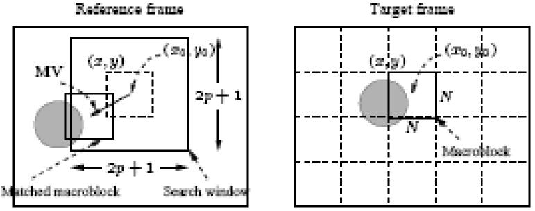
MV search is usually limited to a small immediate neighborhood – both horizontal and vertical displacements in the range [-p,p]. This makes a search window of size (2p+1)(2p+1).
