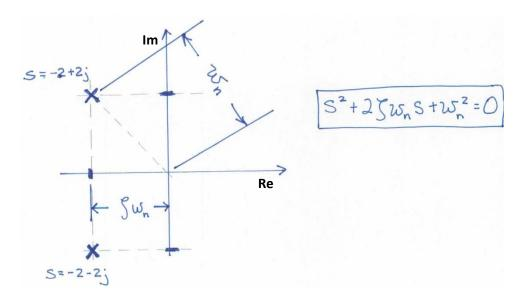
For a simple model of a single-link arm, a control torque,  $\tau$ , is to be used to regulate the angle (i.e., keep it near zero). Assume the dynamics of the system can be modeled as follows:  $mL^2\ddot{\theta} = -B\dot{\theta} - mgLsin\theta + \tau$
