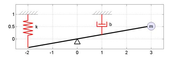
b) Now, solve for  $\omega_n$  and  $\zeta$  numerically, for m=1 (kg), k=900 (N/m), b=36 (N-s/m) and the geometry shown above. (Although you may not know  $r_k$ ,  $r_b$ , and  $r_m$  exactly from the plot, you do know their values *relative* to one another, which is all that is needed to solve the problem.) (*Hint: numbers were picked so math works out "nicely" if you are correct, which may help you catch errors in part a...*)
