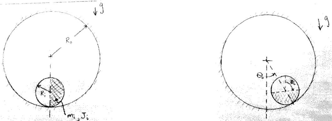
Fig. 2 - The outer perimeter is fixed, and a can rolls freely (without slipping) inside, always touching the perimeter. Definitions for the angle to the point of contact, \theta_o , and the angle of rotation of the can, \phi_i , both of which are measured with respect to an absolute coordinate system, are shown. Shading on the can is only intended to illustrate orientation more clearly: the center of mass is at the center of the can, and the can has mass m_i and inertia J_i .
