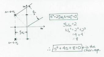
For a simple model of a single-link arm, a control torque, τ, is to be used to regulate the angle (i.e., keep it near zero). Assume the dynamics of the system can be modeled as follows:  $mL^2\ddot{\theta} = -B\dot{\theta} - mgL\sin\theta + \tau$
