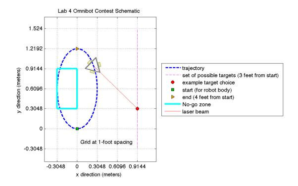
**Figure 1. Schematic for the Omnibot Contest.** Each team must design a controller that will move the omnibot from "start" to "end" while simultaneously pointing a laser at the "target" and avoiding the "no-go zone".
