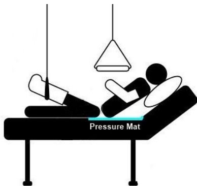
While a patient is lying on a hospital bed, the CuraMat is reading pressure data, converting this data to digital values, and then sending the data wirelessly to a PC
