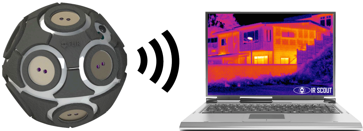
The IR Scout: throw-able, sensor package (left) and the thermal image displayed in full screen mode (right)
