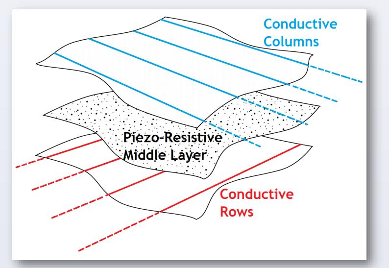
The implemented pressure mat is composed of 50x33 voltage divider circuits. The micro-controllers chooses the circuit via MUXs and DEMUXs and measures the voltage at the pull-down resistor. This voltage is then mapped to pressure.
