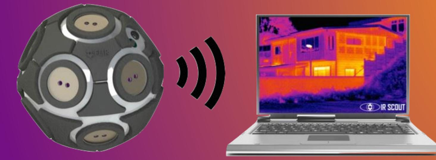
**Throw-able Sensor:** Composed of 12 FLIR Lepton Cameras, an accelerometer, a RN-XV WiFly Module, a Tiva C microcontroller, a TI Fuel Tank Booster Pack, and a 3.7 V Lithium Ion Battery
