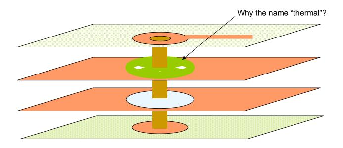
Thermal aperture shown highlighted ... actually it is copper (ORed-in with "+" plane)
