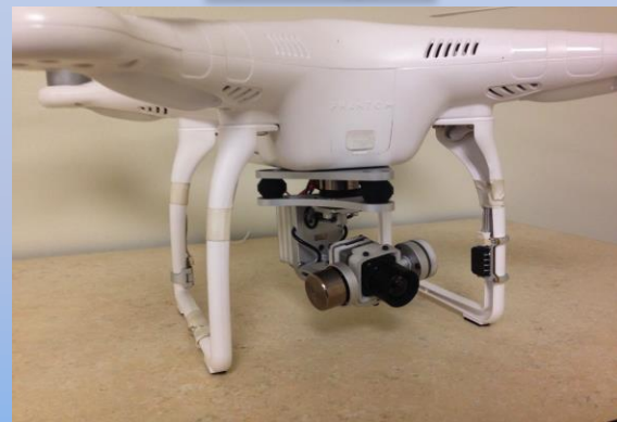
FLIR hummingbIRd mounted to DJI Phantom Drone
