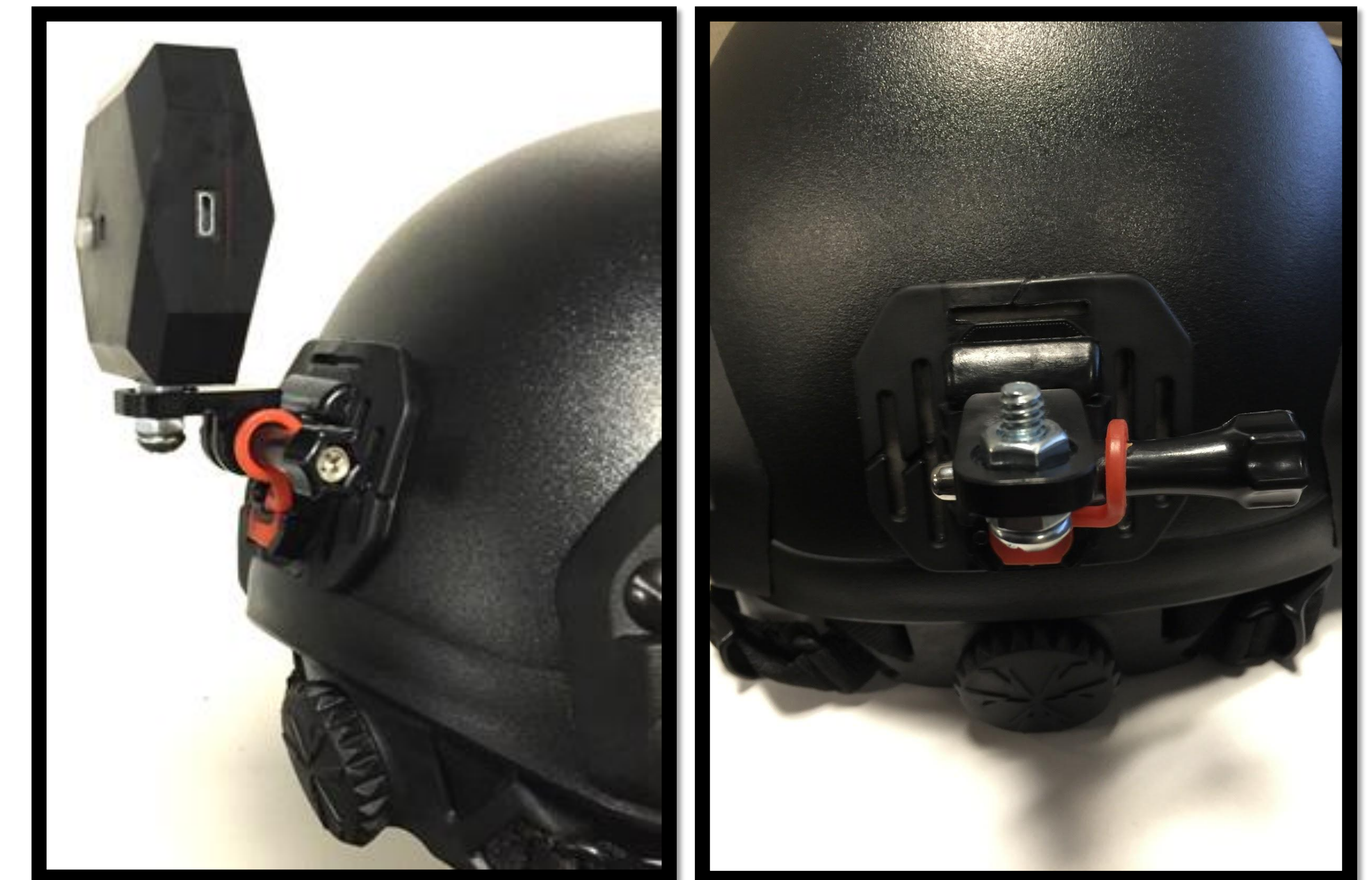
Figure 5: Sensor helmet mounting system.
