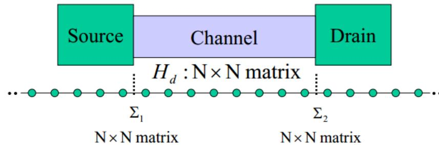
$$\Sigma_1 = \begin{bmatrix} \frac{-e^{ik_1 dx} \hbar^2}{2m^*(dx)^2} & 0 & \dots \\ 0 & 0 & \ddots \\ \vdots & \ddots & \ddots \end{bmatrix} = \begin{bmatrix} -t \exp(ik_1 dx) & 0 & \dots \\ 0 & 0 & \ddots \\ \vdots & \ddots & \ddots \end{bmatrix}$$
