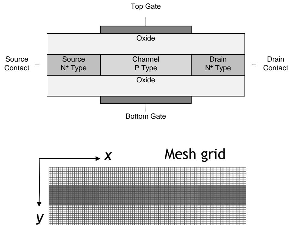
$$\left[ -\frac{\hbar^2}{2m_x^*} \frac{\partial}{\partial x^2} - \frac{\hbar^2}{2m_y^*} \frac{\partial}{\partial y^2} + U(x, y) \right] \psi(x, y) = E \psi(x, y)$$
