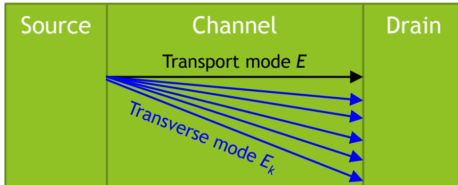
$$F_0(E - \mu) = \sum_{\mathbf{k}} f_0(E + \varepsilon_{\mathbf{k}} - \mu) = S \frac{mk_B T}{\pi \hbar^2} \ln \left( 1 + \exp \left( \frac{\mu - E}{k_B T} \right) \right)$$
