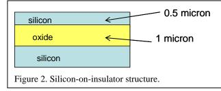
You can form the nanowires by first defining wires (or resistors) in the silicon using diffusion doping and the optical lithography you have used in the lab. Then you can finetune the diameter of the Silicon by *successively oxidizing the wires and selectively etching away the oxide*. Or, you
