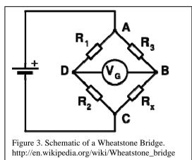
A Wheatstone Bridge is used to make very precise measurements of resistance. An unknown resistance, Rx, can be balanced against three known resistors and the current through the galvanometer,  $V_G$ . Imagine incorporating this Wheatstone Bridge on a silicon chip, with  $R_x$  as a sensor resistor.
