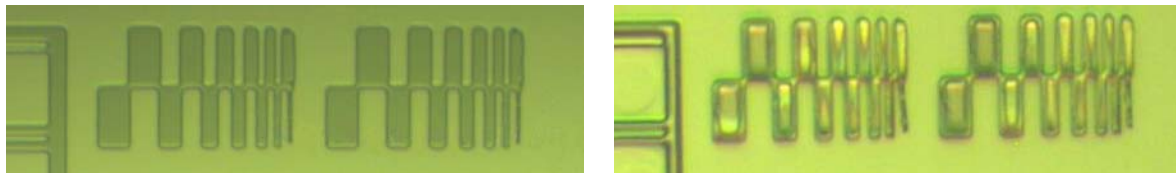
Figure 2. Photoresist exposed for 20 seconds a) before etching b) after etching
