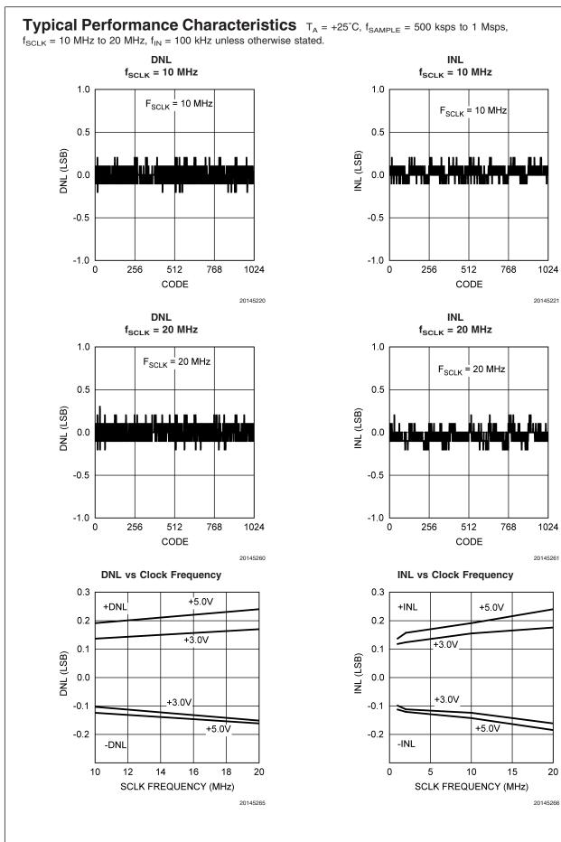
**Typical Performance Characteristics**  $T_A = +25^{\circ}C$ ,  $f_{SAMPLE} = 500$  ksps to 1 Msps,  $f_{SCLK} = 10$  MHz to 20 MHz,  $f_{IN} = 100$  kHz unless otherwise stated. (Continued)
