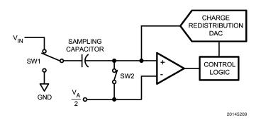
FIGURE 3. ADC101S101 in Track Mode
