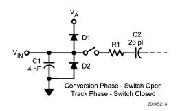
FIGURE 7. Equivalent Input Circuit
