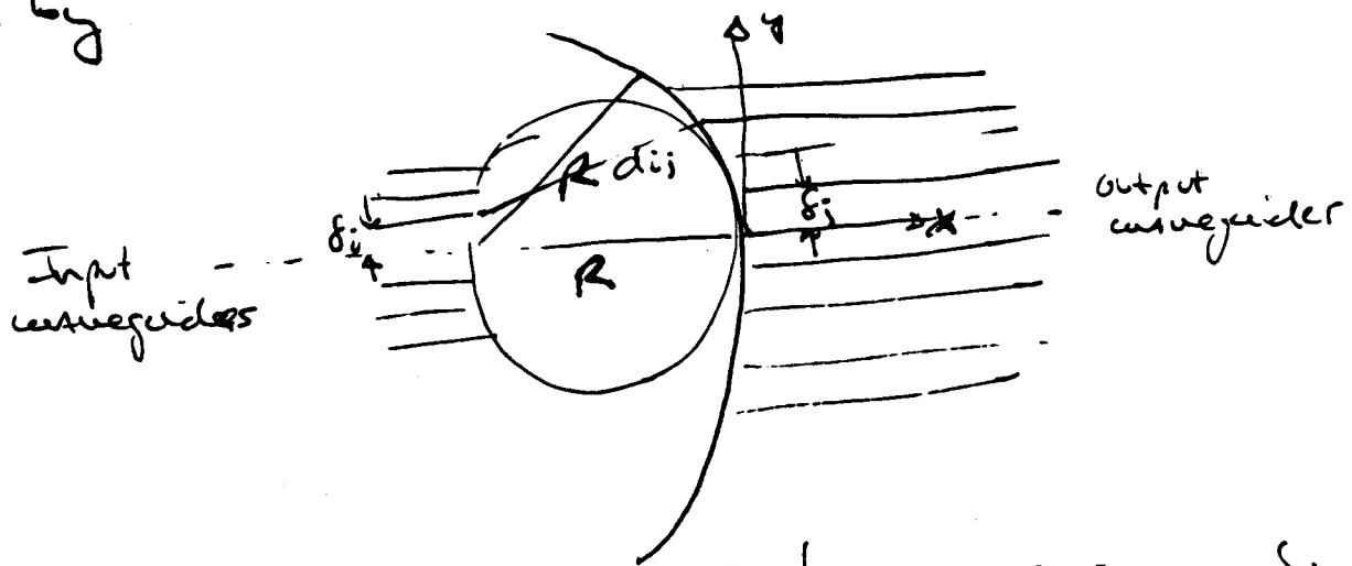
Define offset of input waveguide "i" from  $x$ -axis =  $\delta_i$
