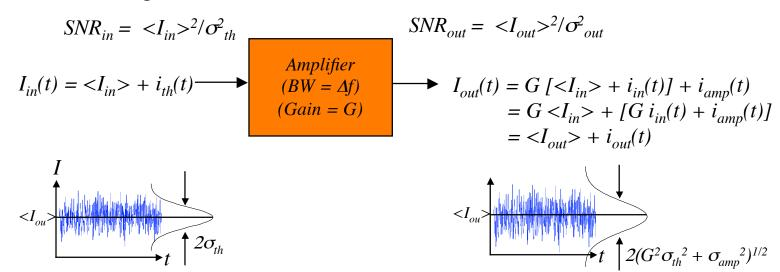
$$F_n = (SNR_{in})/(SNR_{out}) = (\langle I_{in} \rangle^2/\sigma_{th}^2)/(G^2 \langle I_{in} \rangle^2/(G^2\sigma_{th}^2 + G^2\sigma_{eff}^2)) = \sigma_{out}^2/\sigma_{th}^2$$
