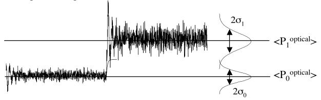
→ OSNR for each level and for complete signal can be defined
