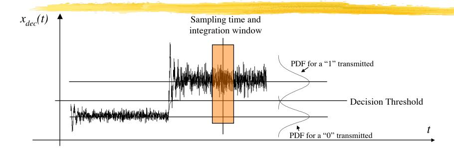
⇒ The bit error rate (BER) of the system depends from the statistics of the resulting noise on the "1" and "0" levels
