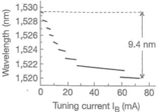
⇒ 3-Section DBR with passive Bragg tuning section
