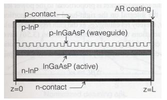
To allow for the presence of gain, we need to modify  $\Delta\beta$  with  $\Delta\beta$  +jg<sub>0</sub>. In this example there are no mirrors, so the matrix F<sub>per</sub> describes the fields and the oscillation condition for lasing is  $(F_{per})_{22} = 0$ .
