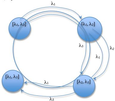
In the case where we need to replace AC and BD by AD and BC, we would need to change the node configurations to the following: Node A -  $[\lambda_1, \lambda_2]$ ; Node B -  $[\lambda_2, \lambda_3]$ ; Node C -  $[\lambda_2, \lambda_3]$ ; Node D -  $[\lambda_1, \lambda_3]$  so that  $\lambda_1$  can be used to setup a lightpath from A to D without blocking any of the other links/lightpaths.
