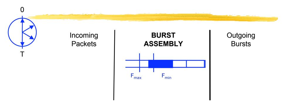
Most bursts exceed  $F_{min}$  before T, but do not reach  $F_{max}$ Normalized burst assembly time  $T_{BN} = 1$ Normalized burst size  $B_N = ICU/7$
