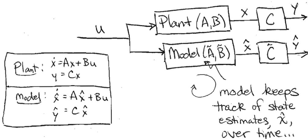
Imagine we have a good idea of the actual plant dynamics. We can run a simulation of what we expect the plant to do,  $\hat{x}$ , along with corresponding, expected output,  $\hat{y}$ .
