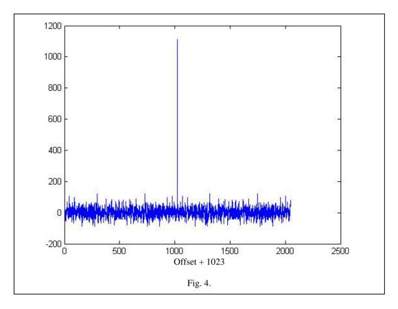
Two key results are obvious from Fig. 4. At zero offset, the autocorrelation indeed shows a peak as one would expect intuitively. And it is even somewhat larger than 1023, representing the fact that the Gaussian statistics allows for fluctuations well beyond the standard deviation (1.0 in the present case). These are clearly evident as the upward or downward going "spikes" in Fig. 3.
