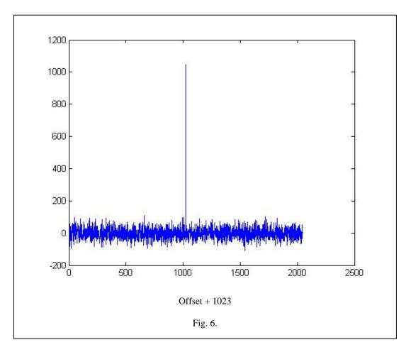
In the language of modern RF systems, this enhancement in SNR between the input and the output of a correlator is called the "processing gain." It presupposes that the correlator is behaving as a matched filter for the signal component of the input waveform, which is generally true of all signals consistent with North's theorem.
