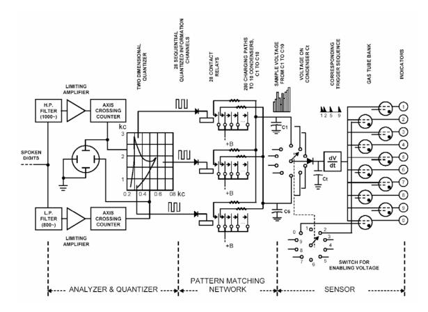
Figure 5 Block schematic of digit recognizer circuits. (Davis, Biddulph, and Balashek [9])
