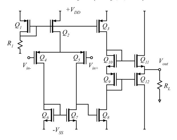
All NMOS:  $I_D = 1(\text{mA/V})(W_g / 1\mu\text{m})(V_{gs} - V_{th} - \Delta V)(1 + \lambda V_{DS})$   $\Delta V = 0.1\text{V}, V_{th} = 0.2\text{V}, 1/\lambda = 5\text{V}$ All PMOS: Also velocity-limited, with  $g_m = 0.5(\text{mA/V})(W_g / 1\mu\text{m})$  $\Delta V = -0.1\text{V}, V_{th} = -0.2\text{V}, 1/\lambda = 5\text{V}$
