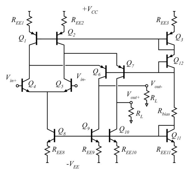
All the transistors have the same (matched)  $I_s$ , have  $\beta = \infty$ , and  $V_A = \infty$  Volts.  $V_{CE(sat)} = 0.5$ V.  $V_{be}$  is roughly 0.7 V, but use  $V_{be} = (kT/q)\ln(I_E/I_s)$  when necessary and appropriate. The supplies are +3.3 Volts and -3.3 Volts. The DC voltage drops across Ree3 and Ree11 are both 300mV.
