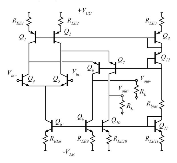
All the transistors have the same (matched)  $I_S$ , have  $\beta=\infty$ , and  $V_A=\infty$  Volts.  $V_{CE(sat)}=0.5 \, {\rm V}$ .  $V_{be}$  is roughly 0.7 V, but use  $V_{be}=(kT/q) \ln(I_E/I_S)$  when necessary and appropriate. The supplies are +4.5 Volts and -4.5 Volts. The DC voltage drops across Ree3 and Ree11 are both 500mV.
