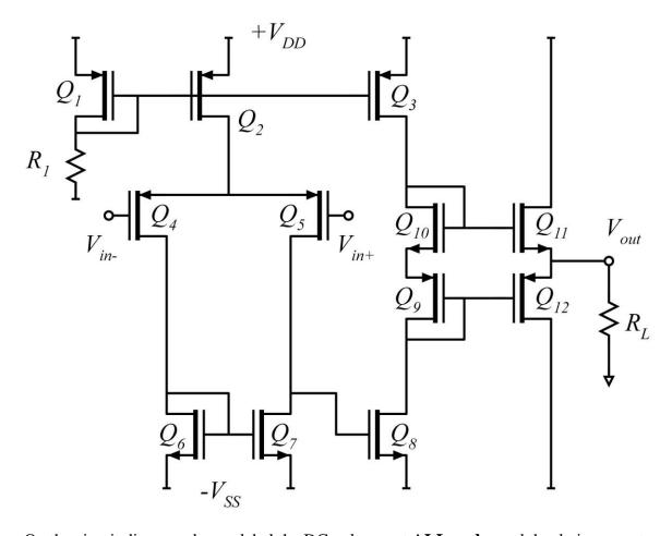
On the circuit diagram above, label the DC voltages at **ALL nodes** and the drain currents of **ALL transistors**
