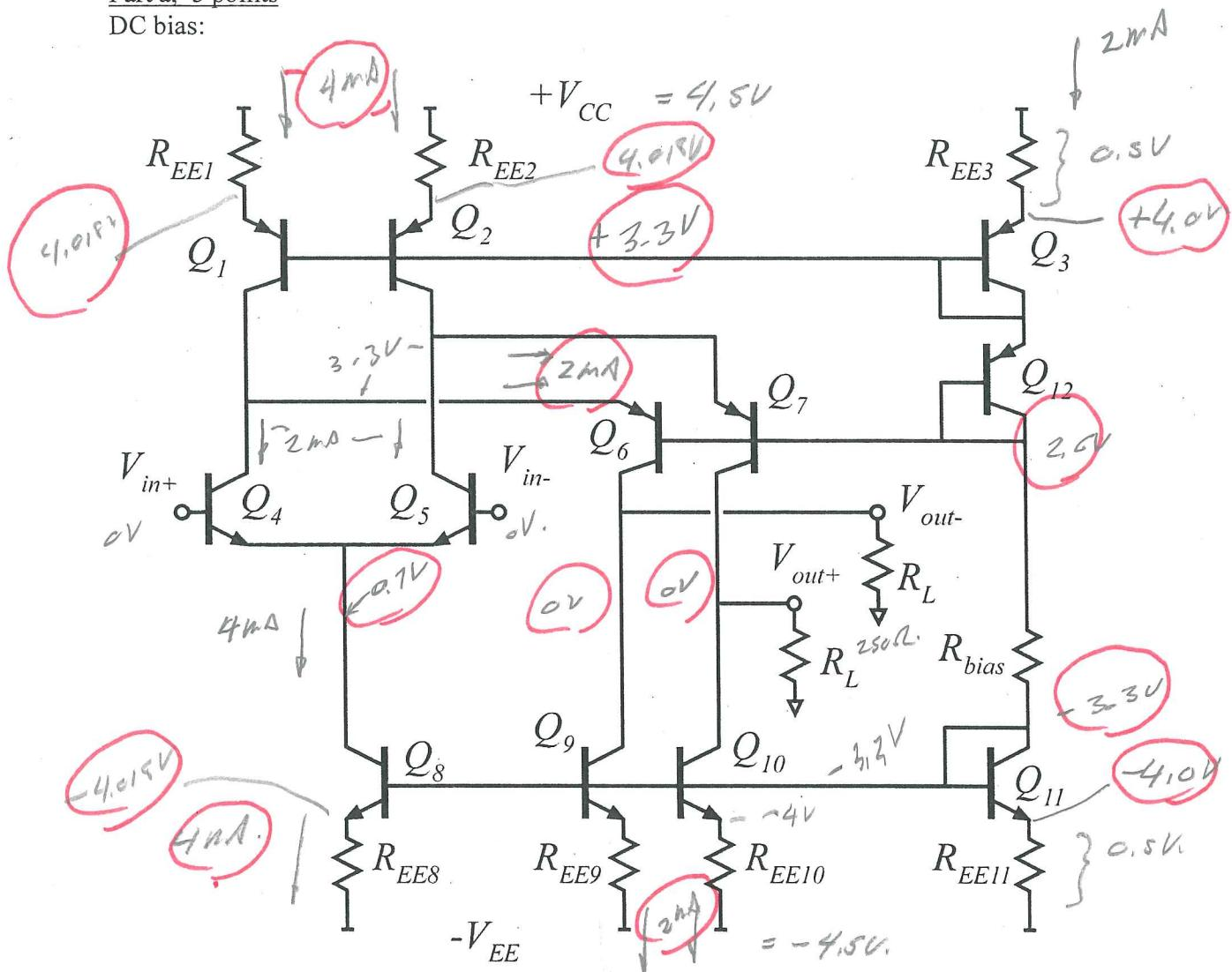
On the circuit diagram above, label the DC voltages at ALL nodes, the DC currents through ALL resistors, and the DC drain currents of all transistors.
