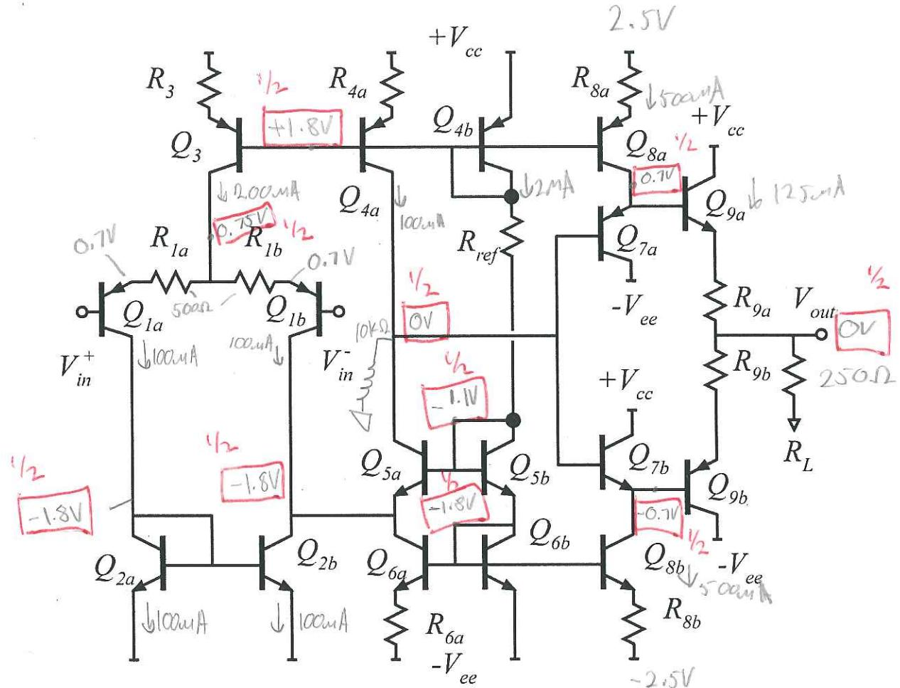
On the circuit diagram above, label the DC voltages at ALL nodes, the DC currents through ALL resistors, and the DC collector currents of all transistors.
