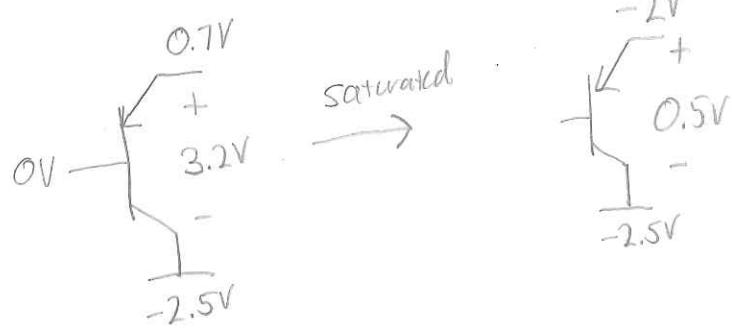
$$\Delta V_{\text{emitter}} = -2.7V$$
