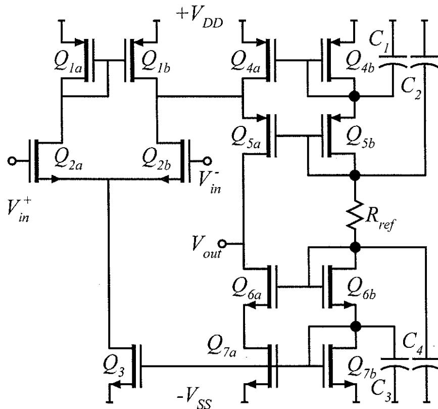
The NMOSFETs and the PMOSFETs have a 0.20 V threshold, a 22nm gate length, 300 cm<sup>2</sup>/Vs mobility, a 10<sup>7</sup>cm/s saturation drift velocity, and  $1/\lambda=3$  Volts. The gate oxide thickness is 1.0nm and the dielectric constant is 3.8. This gives
