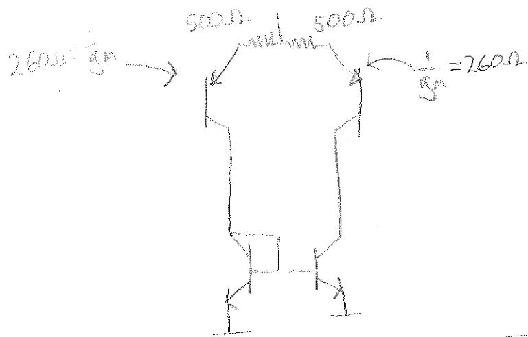
$$\text{Overall transconductance} = \frac{1}{V_{gm1} + R_{ia}} = \frac{1}{500\Omega + 260\Omega} = (760\Omega)^{-1}$$
