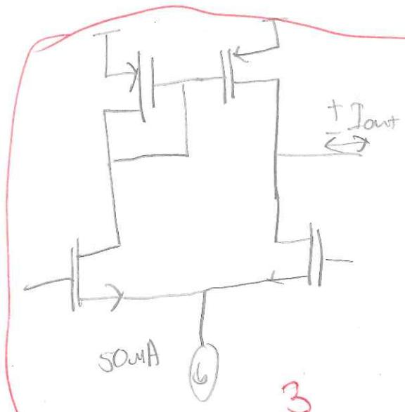
As 2a and 2b are driven, one full-on and the other cut off, I<sub>out</sub> varies by  $\pm 50\text{mA}$
