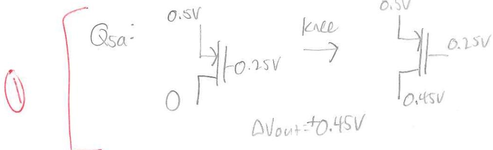
① By symmetry, knee voltage of Q6a limits  $\Delta V_{out}$  to  $-0.45V$
