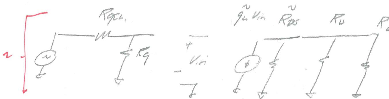
$$\begin{aligned} \boxed{2} \quad g_m &= \frac{g_m}{1 + g_m R_{SAC}} = \frac{1}{1/g_m + R_{SAC}} = \frac{1}{30.4\Omega + 10\Omega} \\ &= \frac{1}{40.4\Omega} \end{aligned}$$
