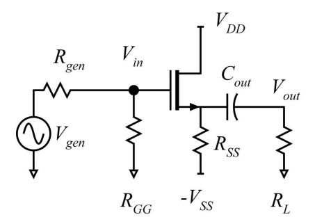
On the circuit diagram above, label the DC voltages at  $\pmb{ALL}$  nodes and the DC currents through  $\pmb{ALL}$  resistors
