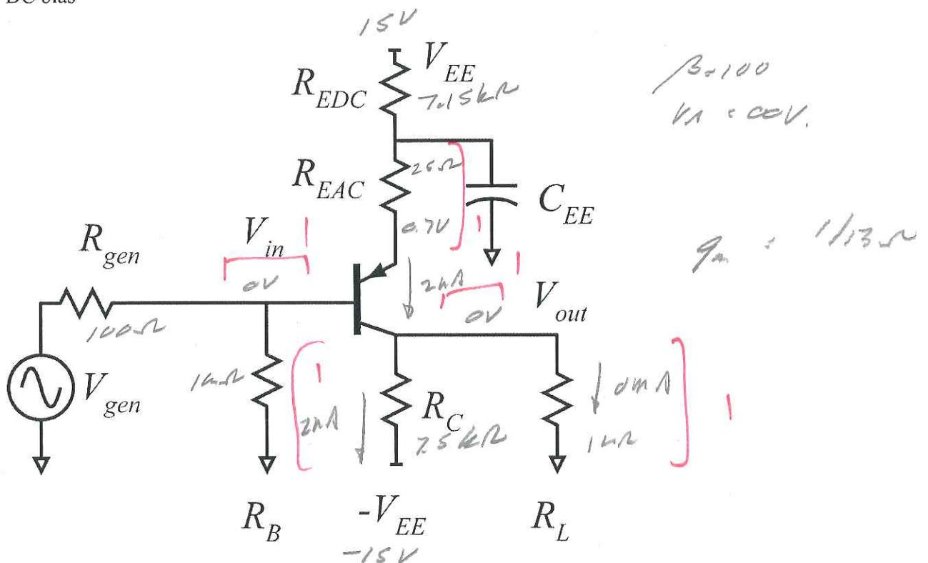
On the circuit diagram above, label the DC voltages at **ALL nodes** and the DC currents through **ALL resistors**
