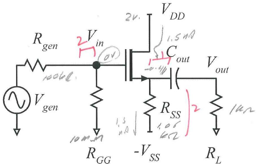
On the circuit diagram above, label the DC voltages at **ALL nodes** and the DC currents through **ALL resistors**
