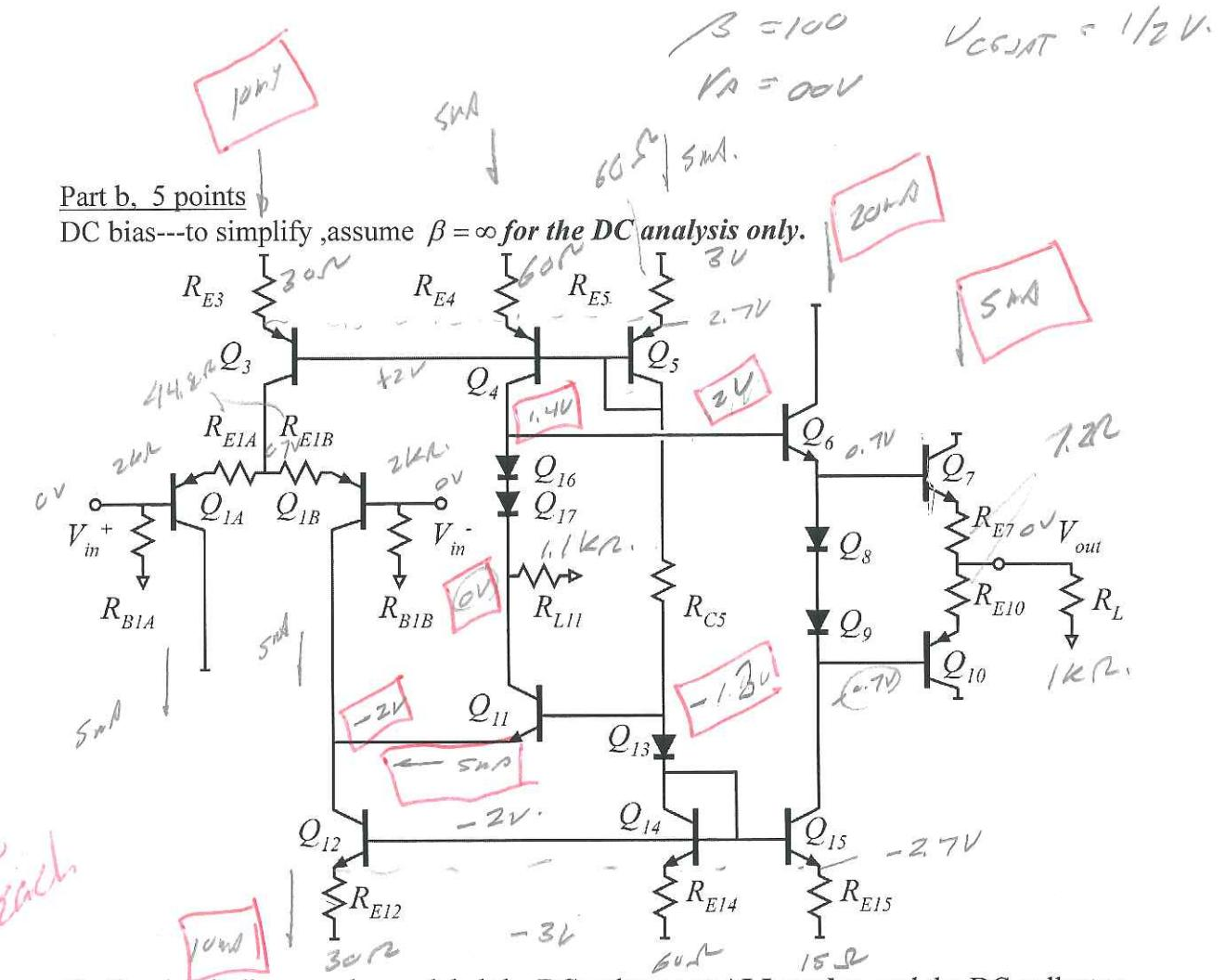
On the circuit diagram above, label the DC voltages at **ALL nodes**, and the DC collector currents of **all transistors**. Label the values of all resistors (except RC5).
