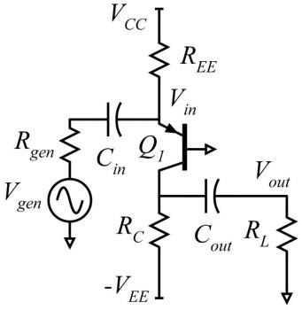
Q1:  $\beta = 100$ ,  $V_A = \text{infinity V, Vce,sat} = 0.5 \text{V}$
