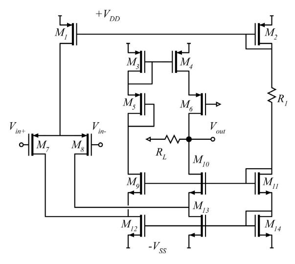
The NMOSFETs have  $K_{\mu} = \mu c_{gs} W_g / 2L_g = 10 \text{mA/V}^2 \cdot (W_g / 1 \mu \text{m})$
