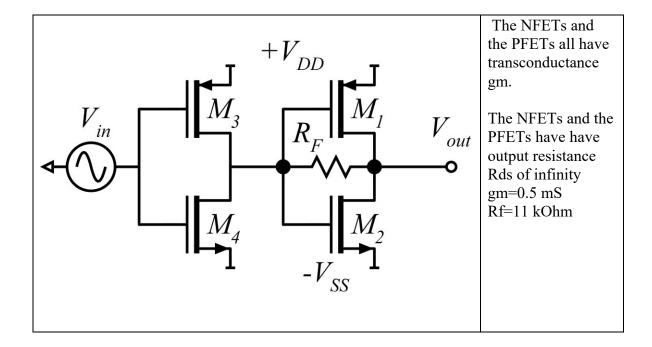
Compute, from nodal analysis, the small-signal gain Vout/Vin. This is a voltage gain. Hint: you can save some work by using the result from part A.
