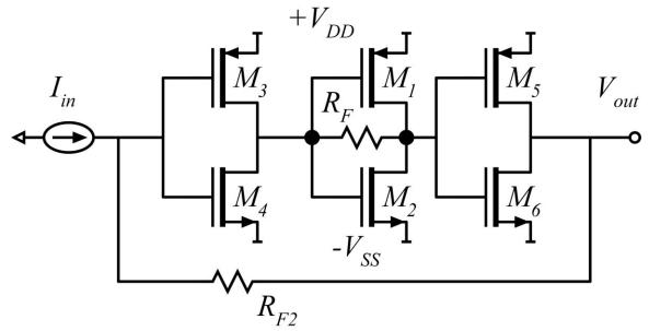
The NFETs and the PFETs all have transconductance gm. The NFETs and the PFETs have have output resistance Rds of infinity. gm=0.5 mS, Rf=11 kOhm, Rf2=1 kOhm.
