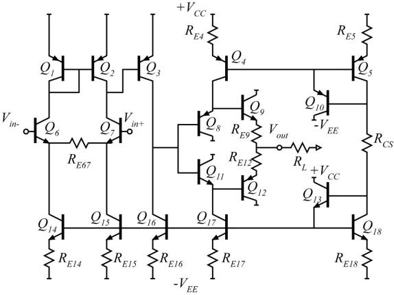
All the transistors have the same (matched)  $I_S$ , have  $\beta = 100$ , and  $V_A = *infinity* Volts$ .  $V_{CE(sat)} = 0.5 \text{V}$ .  $V_{be}$  is approximately 0.7 V, but use  $V_{be} = (kT/q) \ln(I_E/I_S)$  when necessary or appropriate. The supplies are +3 Volts and -3 Volts. All transistors have the same  $I_S$ .
