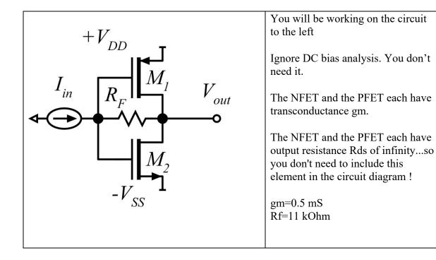
Compute, from nodal analysis, the small-signal gain Vout/Iin. This is called a transimpedance gain.
