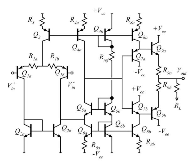
All the transistors have the same (matched)  $I_s$ , have  $\beta = 100$ , and  $V_A = \infty$  Volts.  $V_{CE(sat)} = 0.5$ V.  $V_{be}$  is roughly 0.7 V, but use  $V_{be} = (kT/q)\ln(I_E/I_s)$  when necessary and appropriate. The supplies are +2 Volts and -2 Volts.
