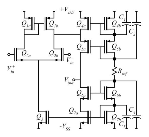
The NMOSFETs and the PMOSFETS have a 0.20 V threshold, a 22nm gate length, 300 cm<sup>2</sup>/Vs mobility, a  $10^7$  cm/s saturation drift velocity, and  $1/\lambda = 3$  Volts. The gate oxide thickness is 1.0nm and the dielectric constant is 3.8. This gives
