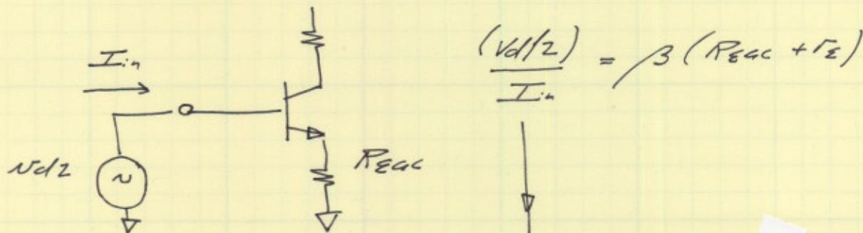
$$\begin{aligned} V_{d1/2}/I_{in} &= 2/\beta (r_e + R_{EAC}) \\ &= R_{in, \text{differential}} \end{aligned}$$
