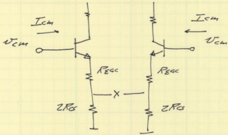
$$\frac{V_{cm}}{I_{cm}} = \beta (\tau_e + R_{ECC} + Z_{RCS}) \approx 2\beta R_{CS}$$
