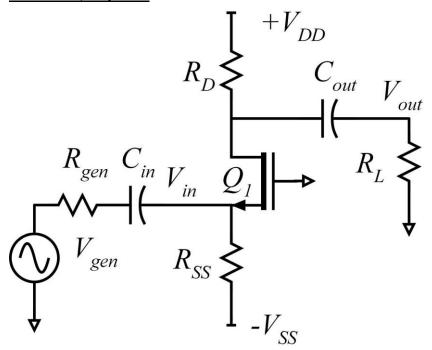
Q1 has 1.0 nm oxide thickness,  $\varepsilon_r$ =3.8, 22 nm gate length, and a 0.2 V threshold. Mobility is 400 cm^2/(V-s), saturation drift velocity is 1E7 cm/s,  $\lambda$  = 0 Volts<sup>-1</sup>,  $C_{gs} = \varepsilon_r \varepsilon_{ox} L_g W_g / T_{ox} + (0.5 \mathrm{fF} / \mu \mathrm{m}) \cdot W_g$  and  $C_{gd} = (0.5 \mathrm{fF} / \mu \mathrm{m}) \cdot W_g$ . Hints:
