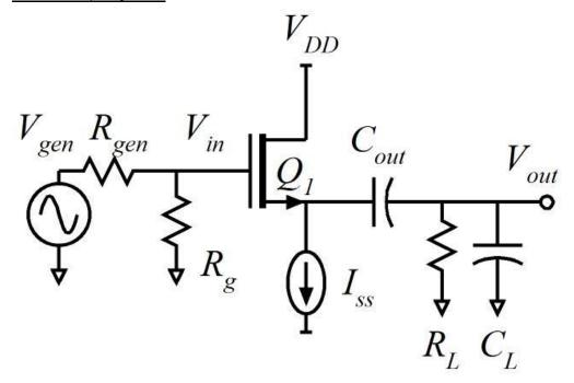
Q1 has 0.9 nm oxide thickness,  $\varepsilon_r$ =3.8, 12 nm gate length, and a 0.2 V threshold. Mobility is 400 cm^2/(V-s), saturation drift velocity is 1E7 cm/s,  $\lambda$  = 0 Volts<sup>-1</sup>,  $C_{gs} = \varepsilon_r \varepsilon_{ox} L_g W_g / T_{ox} + (0.5 \text{fF} / \mu \text{m}) \cdot W_g$  and  $C_{gd} = (0.5 \text{fF} / \mu \text{m}) \cdot W_g$ . calculated for you:
