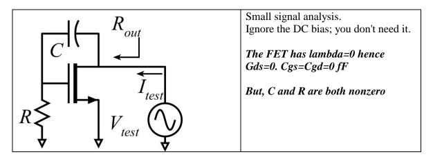
Replacing the transistor with its high frequency small-signal model, draw a small-signal equivalent circuit diagram.
