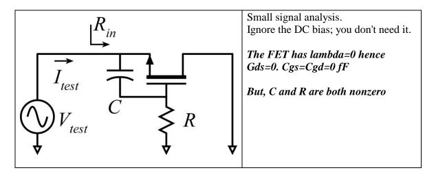
Replacing the transistor with its high frequency small-signal model, draw a small-signal equivalent circuit diagram.
