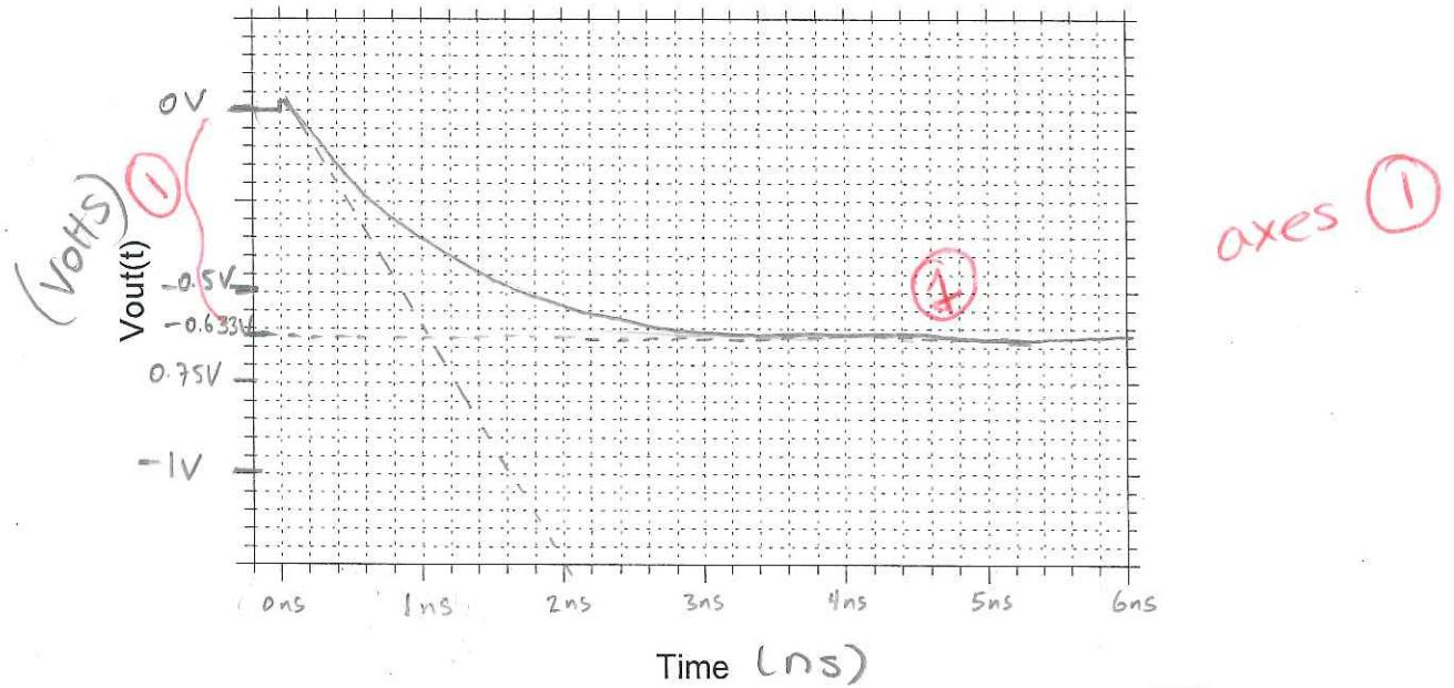
$$V_{in}(+) = 0.1V u(t) \Rightarrow V_{in}(s) = \frac{0.1V}{s} \quad ①$$
