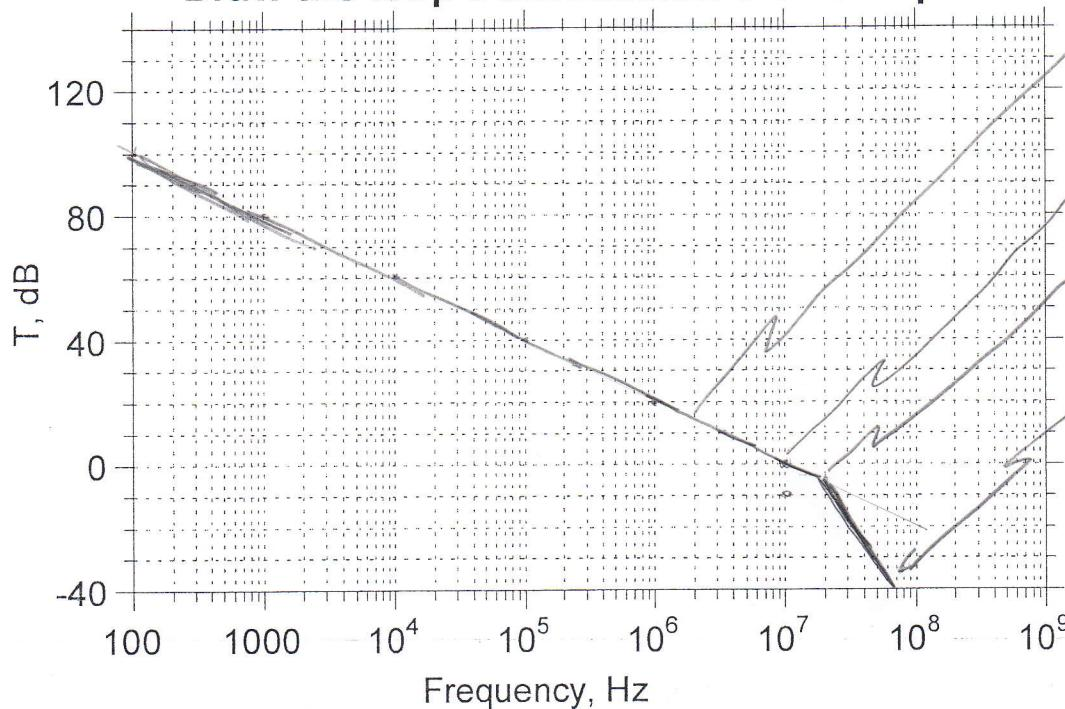
$$\begin{aligned} \text{LT @ } f_{loop} &= -90^\circ - \arctan\left(\frac{10 \text{ mHz}}{20 \text{ mHz}}\right) \\ &= -90^\circ - 26.6^\circ \\ \text{phase margin} &= 90 - 26.6 = \underline{\underline{33.4^\circ}} \end{aligned}$$
