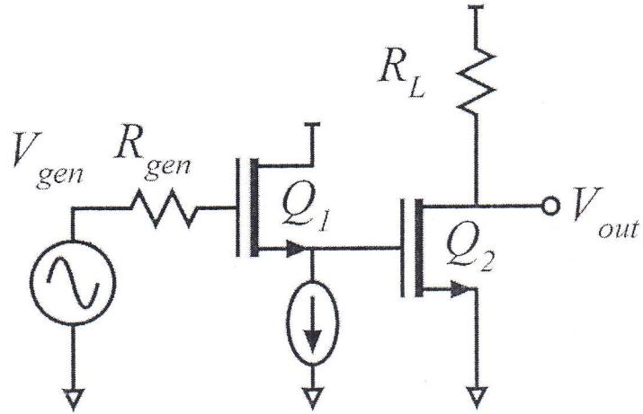
In the circuit above  $g_{m1} = 10 \text{ mS}$ ,  $g_{m2} = 50 \text{ mS}$ .
