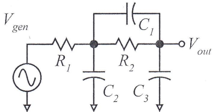
$$\frac{V_{out}}{V_{gen}} \Big|_{DC} = \frac{1}{1 + a_1 s + a_2 s^2}, \quad a_1 = \frac{1}{2 \mu s}, \quad a_2 = \frac{1.1 \cdot 10^{-11} \text{ See}^2}{1 \mu s}$$
