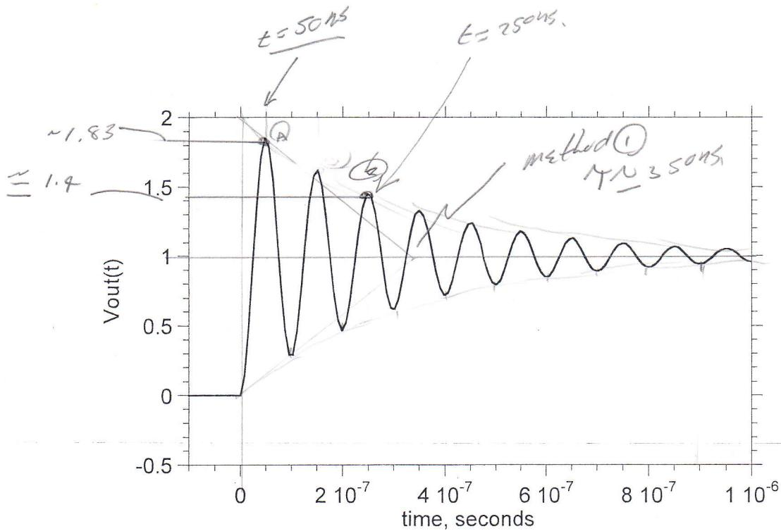
Determine the frequency and damping factor of the dominant poles of the transfer function.
