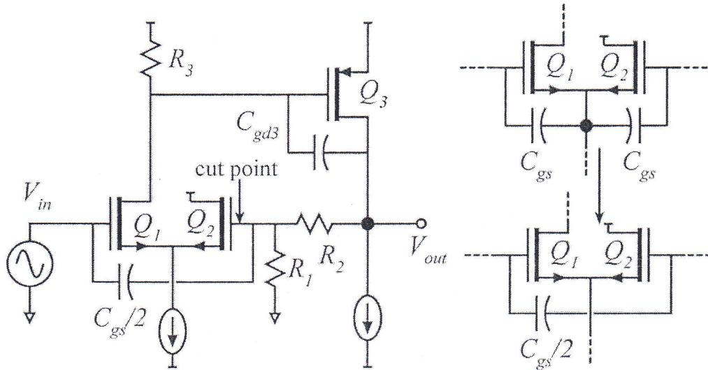
In the circuit above  $g_{m1} = g_{m2} = 20 \text{ mS}$ ,  $g_{m3} = 100 \text{ mS}$ ,  $R_1 = 1 \text{ k}\Omega$ ,  $R_2 = 9 \text{ k}\Omega$ .
