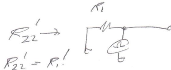
$\rightarrow R_{11}^0 C_1 C_2 R_{22}' = 1\mu\text{s} \cdot (2\text{nF}) 1\text{k}\Omega = 1\mu\text{s} \cdot 2\mu\text{s}$
