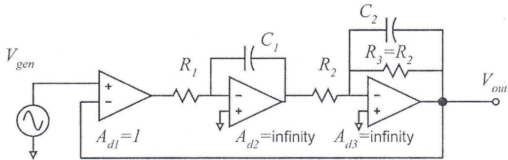
In the circuit above,  $A_{d2}$  and  $A_{d3}$  are ideal, infinite-gain op-amps.
