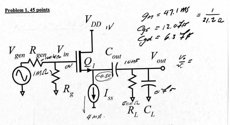
Q1 has 0.9 nm oxide thickness,  $\varepsilon_r = 3.8$ , 12 nm gate length, and a 0.2 V threshold. Mobility is 400 cm<sup>2</sup>/(V-s), saturation drift velocity is 1E7 cm/s,  $\lambda = 0$  Volts<sup>-1</sup>,  $C_{gs} = \varepsilon_r \varepsilon_{ox} L_g W_g / T_{ox} + (0.5 \text{fF} / \mu \text{m}) \cdot W_g$  and  $C_{gd} = (0.5 \text{fF} / \mu \text{m}) \cdot W_g$ . calculated for you:
