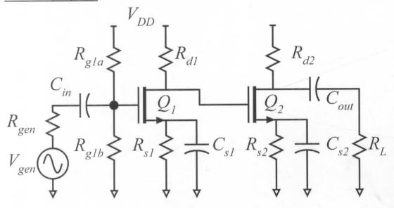
In the amplifier above, Rgen=100kOhm, Rg1a=Rg1b=500kOhm, Rs1=Rs2=100 Ohms. VDD=5Volts gm1=5 mS, gm2=10mS Rd1=1 kOhm, Rd2=2kOhm, RL=10kOhm. Cin, Cout, Cs1, Cs2 are all very large Cgs1=0fF, Cg1d=5fF, Cgs2=20 fF, Cgd2=0fF Gds1=Gds2=0mS
