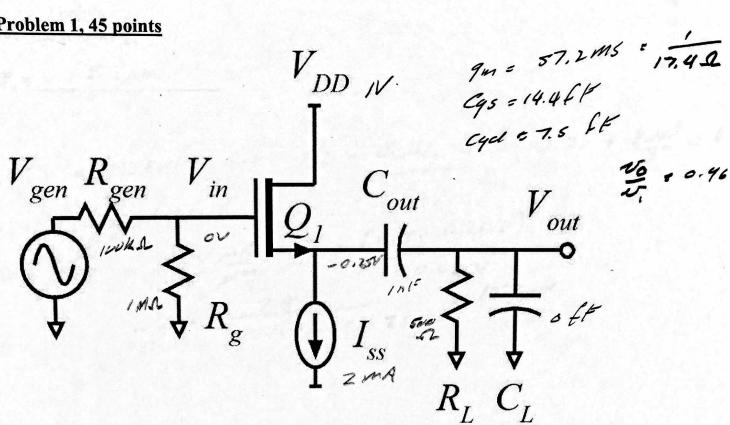
Q1 has 0.9 nm oxide thickness,  $\varepsilon_r$ =3.8, 12 nm gate length, and a 0.2 V threshold. Mobility is 400 cm<sup>2</sup>/(V-s), saturation drift velocity is 1E7 cm/s,  $\lambda = 0$  Volts<sup>-1</sup>,  $C_{gs} = \varepsilon_r \varepsilon_{ox} L_g W_g / T_{ox} + (0.5 \text{fF} / \mu \text{m}) \cdot W_g \text{ and } C_{gd} = (0.5 \text{fF} / \mu \text{m}) \cdot W_g$ . calculated for you:
