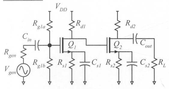
In the amplifier above, Rgen=100kOhm, Rg1a=Rg1b=500kOhm, Rs1=Rs2=100 Ohms. VDD=5Volts gm1=5 mS, gm2=10mS Rd1=1 kOhm, Rd2=2kOhm, RL=10kOhm. Cin, Cout, Cs1, Cs2 are all very large Cgs1=0fF, Cg1d=5fF, Cgs2=0 fF, Cgd2=10fF Gds1=Gds2=0mS
