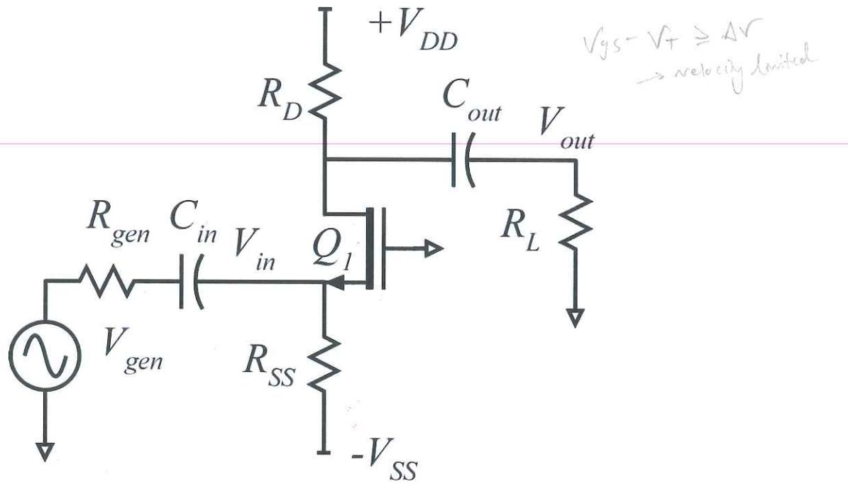
Q1 has 1.0 nm oxide thickness,  $\epsilon_r = 3.8$ , 22 nm gate length, and a 0.2 V threshold.
