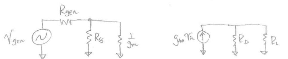
$$\begin{aligned} R_{gen} &= 50\Omega \\ R_{ss} &= 1760\Omega \\ R_D &= 1000\Omega \\ R_L &= 3000\Omega \\ \frac{1}{g_m} &= 20.0243\Omega \end{aligned}$$
