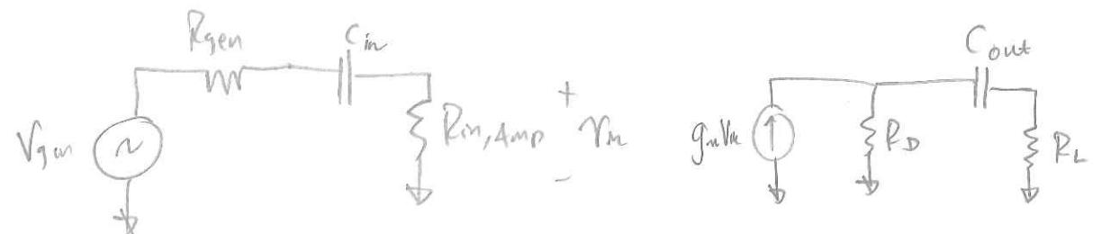
$$\begin{aligned} T_{in} &= (R_{gen} + R_{in,Amp}) C_{in} \\ &= (50\Omega + 19.8\Omega) (1\text{nF}) \end{aligned}$$
