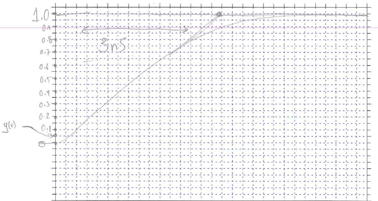
$$H(s) = (10) \frac{1 + s(200\mu s)}{1 + s(3\mu s)} \quad X(s) = (100mV) \left(\frac{1}{s}\right)$$
