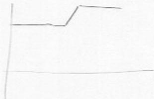
4) zero @  $f_{z1} = \frac{0.159}{2 \text{ ms}} = 79.5 \text{ Hz.}$
