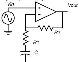
The differential amplifier has infinite differential input impedance and zero output impedance. Its low-frequency gain is 10<sup>6</sup>, and it has a single pole in its transfer function at 2 Hz.
