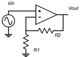
The amplifier has a differential gain of  $10^7$ . R1=1 kOhm, R2=19 kOhm. The op-amp has infinite differential input impedance and zero differential output impedance.
