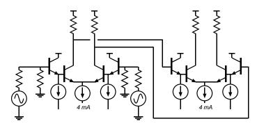
A basic differential video amplifier is shown on the left. This circuit is fully differential, and so can be analyzed by the half-circuit method, where the connected emitters of the differential pairs become virtual grounds.
