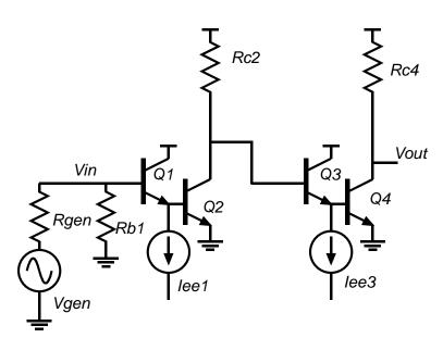
The circuit we therefore analyze is to the left. This is an AC equivalent circuit: It does not represent the DC.
