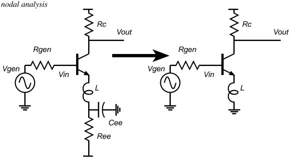
Inductance, often present in the emitter lead of a common-emitter amplifier, can have a serious effect on high frequency response. Working from the small-signal equivalent *circuit on the right*, with Rgen=*zero* Ohms, Rc=100 Ohms, L=1 nH, re=26 Ohms, Cbe=1 pF, Ccb=0pF, beta=infinity, Va=infinity, find Vout/Vgen by nodal analyis. Give
