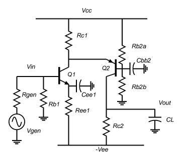
In the circuit, the power supplies are +/- 10 volts. The transistors have beta=1000, ft=1 GHz, and Ccb=0.5 pF. CL=1 pF. Va=infinity.
